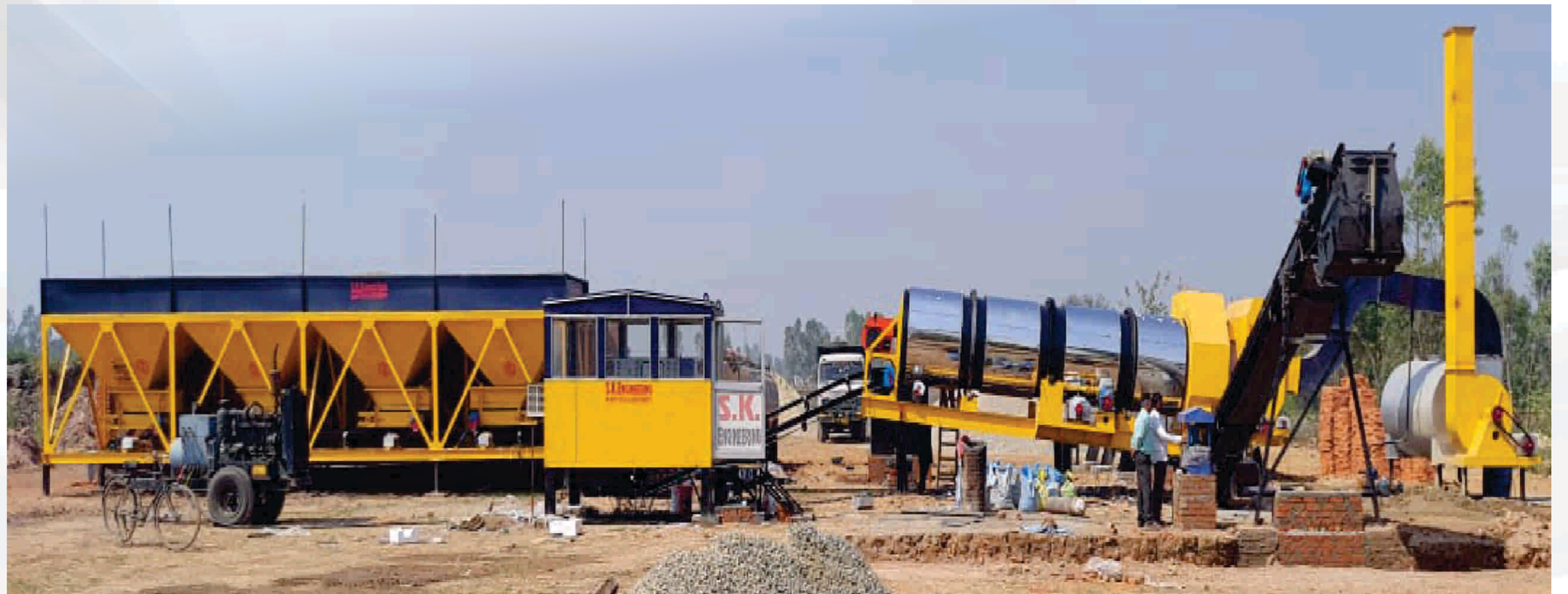
ASPHALT HOT MIX PLANT LAYOUT
